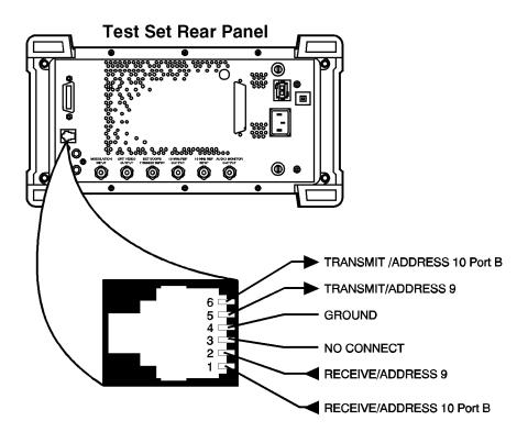
Figure 1 Test Set RJ-11 Serial Port Connections
