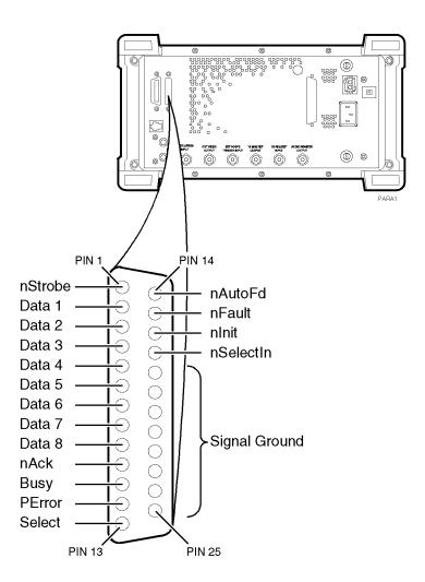
Figure 2 Test Set Parallel Port Connections
