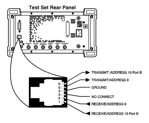
Figure 3 Test Set RJ-11 Serial Port Connections
